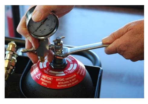
caution must be taken to avoid overtightening. Overtightening the swivel assembly may result in damage to the bladder valve assembly, causing it to leak.
