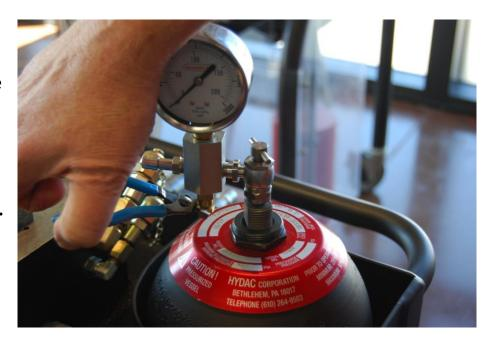
trapped gas pressure in the charging hose after the bladder is charged and prior to removing the hose.)
